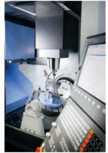
The DVF 5000 is designed to machine complex work pieces with high precision and speed. The 18,000 RPM built-in spindle gives superior performance in virtually any machining application. The travelling column machine structure provides uniform load to all linear machine axes allowing for a highly rigid and stable platform for your most demanding machining processes.
