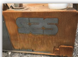
Barge in Gulf of Mexico, coated sections protected after 1 year
