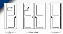
Just as in the modular design of the AccuCab and Hybrid AccuCab, the WeighStation™ allows for single or double cabinet configuration and comes standard with wheels and feet for easy movement. The clear pull-out shelving offers easy access and the shelf placement is customizable providing ample space to house inventory stored in various sized-weight sensing bins.
